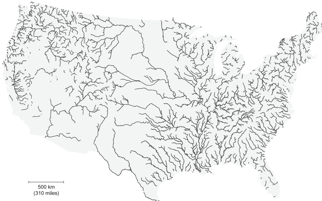
Figure 12. Conterminous United States, approximately 1:10M scale. Pruning threshold (cfs) = 0.001 \times \text{precipitation (mm} \times 100) .
