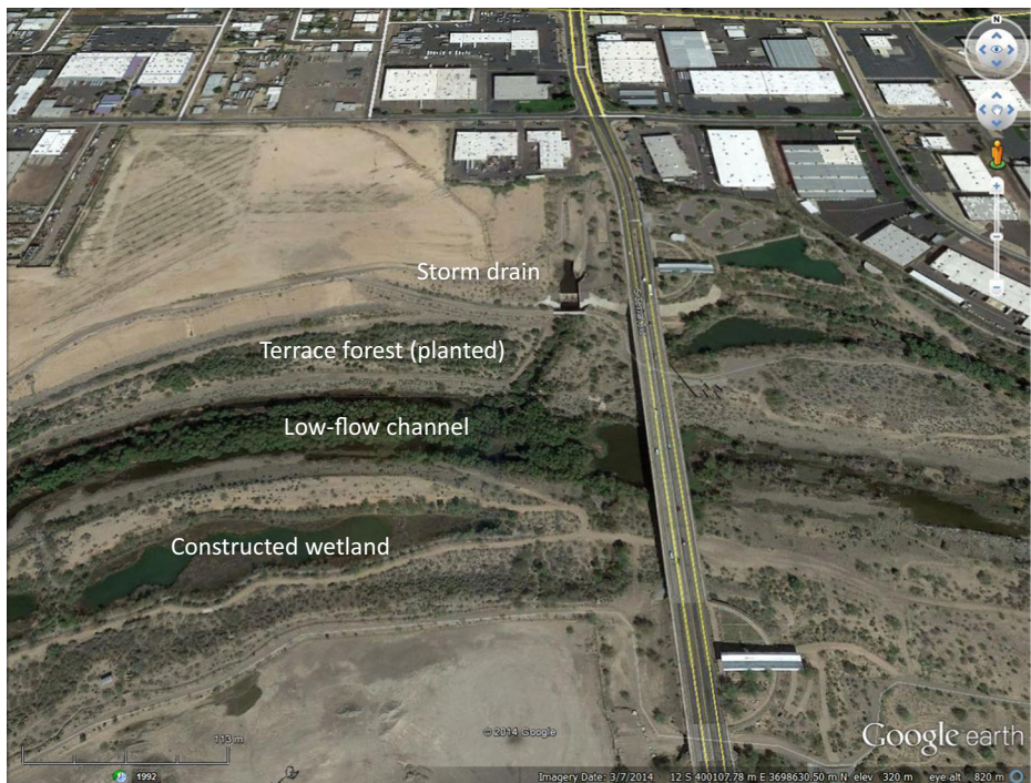
Fig. 4 A restored section of the Salt River (Phoenix Rio Salado) showing landscape features within the riparian zone
