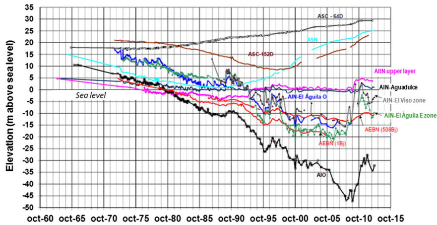
Fig. 8. Piezometric level evolution in some wells in the Campo de Dalías aquifer. Drawdown is continuous in the intensively exploited deep aquifers, while in the almost unexploited upper aquifers water levels go up due to increased recharge from loses in the water distribution network for irrigation and return irrigation flows. The final trend to recovery is due to the extraordinary wet 2009–2011 period, during which recharge in the Sierra de Gádor aquifers increased and decreased water demand. Modified after Domínguez-Prats et al. (2013).
