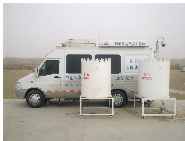
Figure 2. CFL-03 mobile boundary layer wind-profiling radar in operation in the central Taklamakan Desert.
