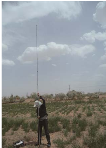
Fig. 2 The process of soil sampling with Luoyang shovel. For sampling soil in the depth profiles, a customized auger (traditionally, Luoyang shovel) with detachable 0.5-m steel tubes which can be assembled to 5-m was employed.
