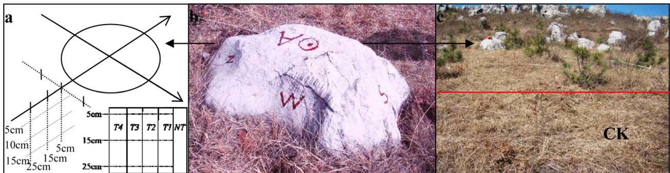
Fig. 2 Illustration of bare rock outcrops at the investigated site a schematic map of individual rock samples for soil moisture measurement at different distances and depth; b rock sample A (see Fig. 1); c control plot CK. (Modified after Li et al. 2014)
