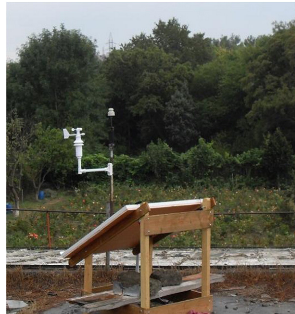
Fig. 2. Condenser and its weather station.
