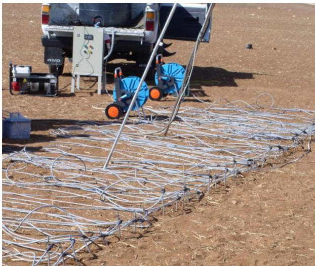
Fig. 4 Setup of high resolution resistivity imaging survey intended to calibrate rain simulation
