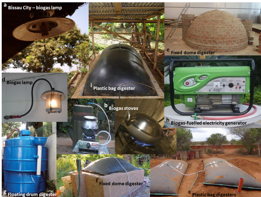
Fig. 2 Examples of small-scale low-tech AD proposed by various experiences worldwide, biogas-fed stove, lamps and biogas-fuelled electric power generator. a Original photo shoot; b CSIR (2014); c http://blog.wildlifeworks.com/ ; d http://portfolio.co.ke/article/from-the-dung-pit-to-the-kitchen-the-biogas-myth/ ; e http://www.heringinternational.co.za/ ; f http://www.homepower.com/ ; g http://www.thehindu.com/ ; h www.acmeagro.org ; i http://agroindustriindonesia.blogspot.it/
