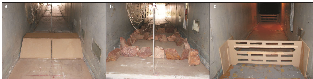
Fig. 4 Experimental models in wind tunnel. a, railway embankment model; b, SCB model; and c, SF model
