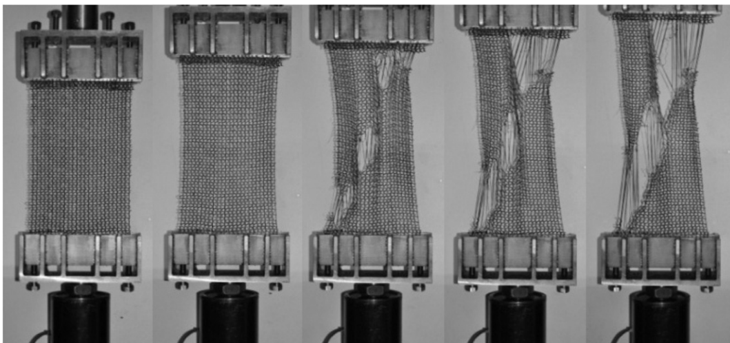
Fig. 5. Tensile test of Raschel mesh with 35% shade coefficient along the longitudinal direction. Maximum force is reached in the third photo from the left.
