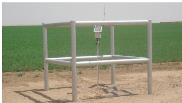
Fig. 4 The EnviroSCAN multilevel soil moisture sensor at pivot no. 26
