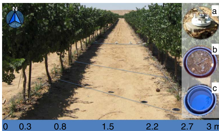
Figure 1. Below canopy measurement setup for intensive observation periods (a) with a row of pyranometers in the back, (b) a row of microlysimeters, and (c) a row of micropans in front.
