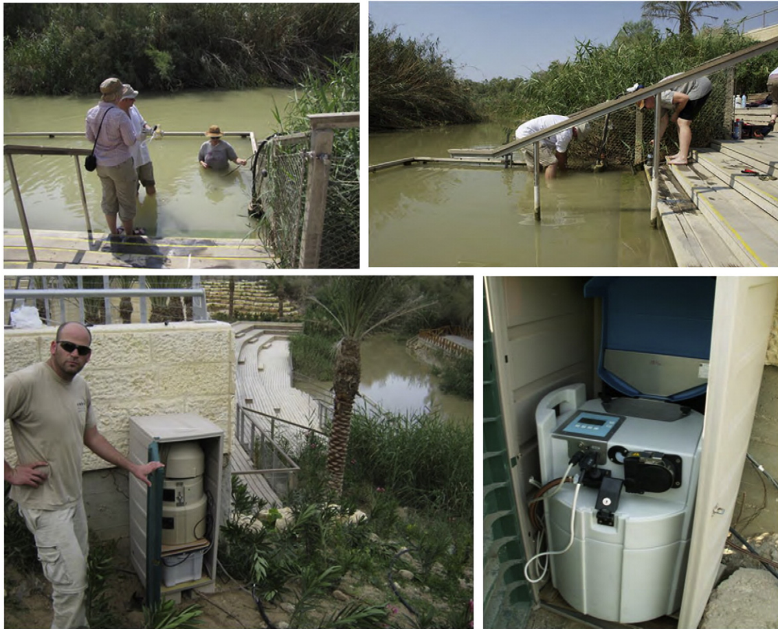
Fig. 5. Installation of the hydrometric station inside the Lower Jordan River at Baptism Site. Sensor installation and view over the river towards Jordan (upper row), hidden sensor logger and auto sampler (lower row).
