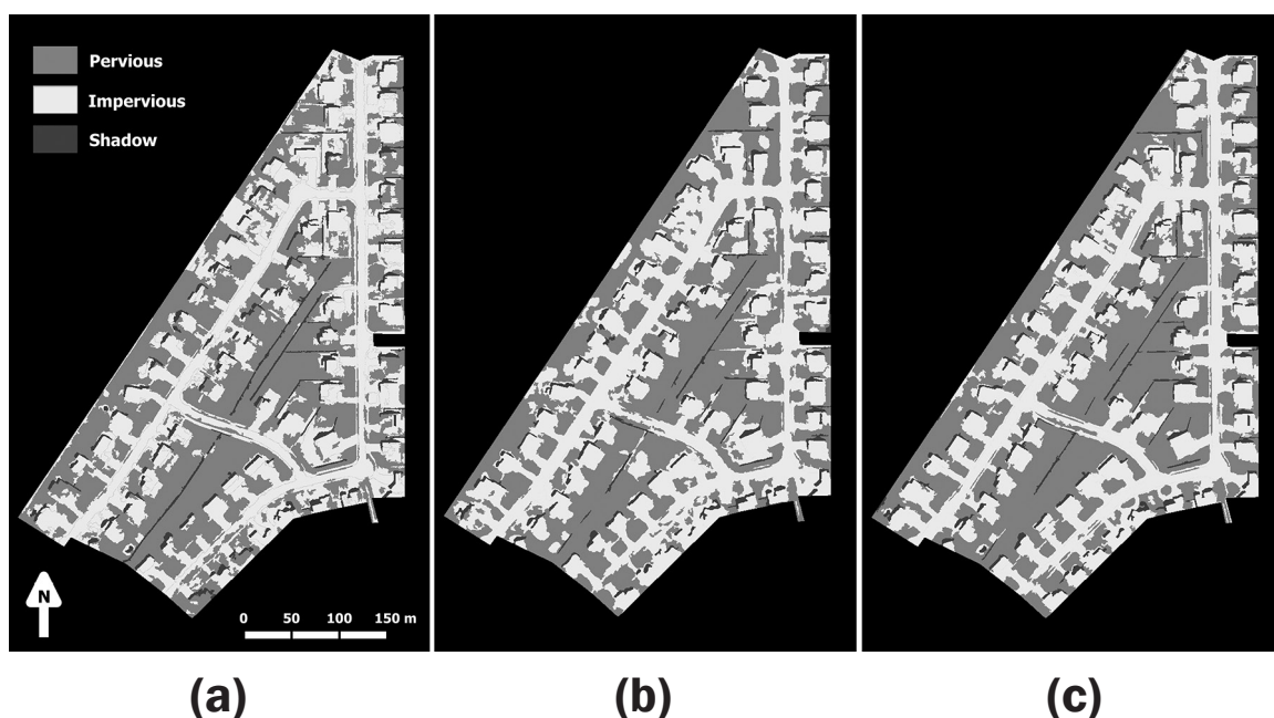
Figure 5. (a) Classification results for the Vis dataset, (b) PCA-Plus dataset, and (c) Pan/Vis/NIR-Plus dataset, where light gray = impervious, middle gray = pervious, and dark gray = shadow.
