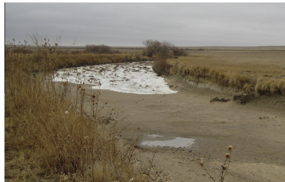
Fig. 2. A wetting front moving down an initially dry channel in eastern Colorado, USA. The speed of the advancing front is sensitive to the hydraulic conductivity of the streambed (and hence the infiltration rate), allowing for this to be calibrated based on observed timings of front arrival along the channel.
