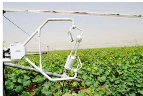
Fig. 1 The eddy covariance (EC) system deployed inside the screenhouse, under the screen and above the table-grape plants
