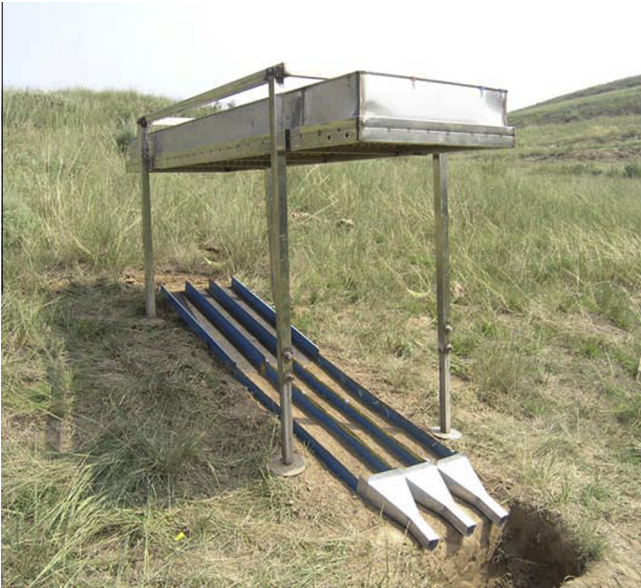
Fig. 2. Photograph of the run off-on-out rainfall simulator used for infiltration test.
