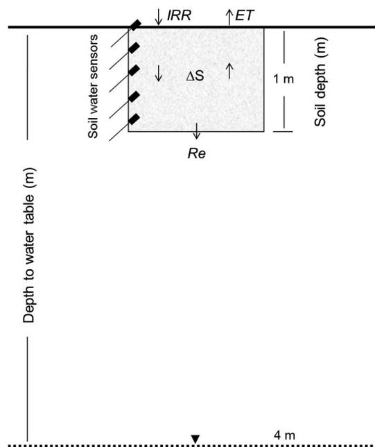
**Fig. 2.** Schematic showing installation of soil water content sensors and the different water budget components used to estimate potential aquifer recharge in the apple orchard
