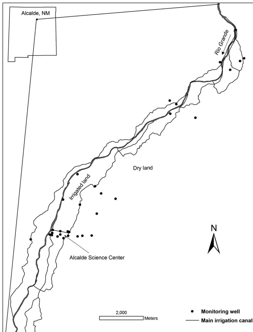
Fig. 1. Map of the study area showing the network of main irrigation canals and monitoring wells used in this study
