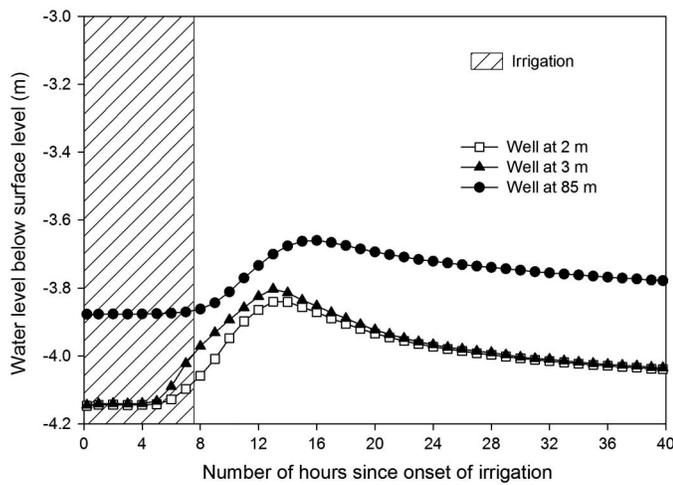
**Fig. 5.** Water table fluctuations in response to irrigation percolation on June 7, 2006, in three wells located at different distances from the water line in the alfalfa-grass field
