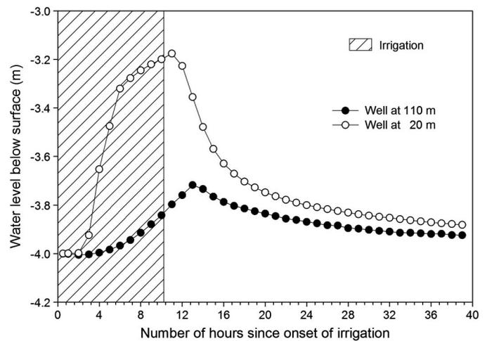
**Fig. 7.** Water table fluctuations in response to irrigation percolation on May 24, 2006, in two wells located at different distances from the water line in the apple orchard
