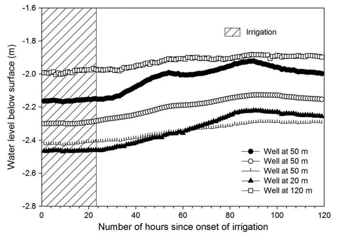
**Fig. 6.** Water table fluctuations in response to irrigation percolation on June 24, 2008, in five wells located at different distances from the water line in the oat-wheatgrass field
