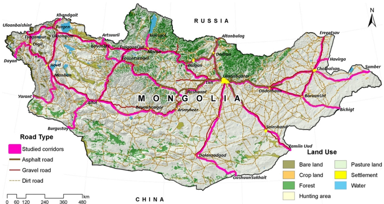
Fig. 4. Arterial routes of Mongolia studied in this analysis overlaid on the land-use map. (Source: Authors' elaboration based on roads dataset from RSRC, 2008).
