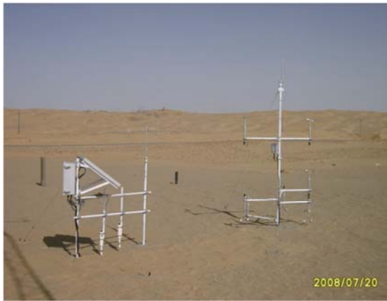
Fig. 2 The 2-m meteorological tower and piezoelectric saltation sensors (Sensit)
