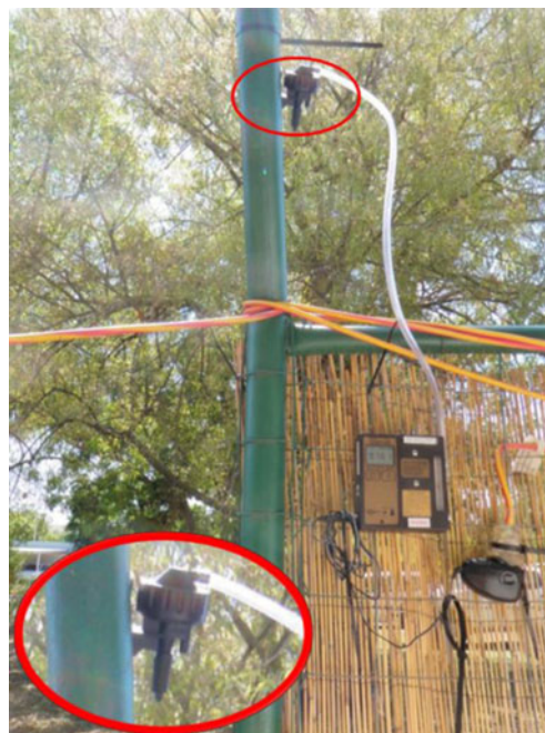
Fig. 2 SKC® cyclone and sampling configuration in the backyard of a house for outdoor PM 10 collection
