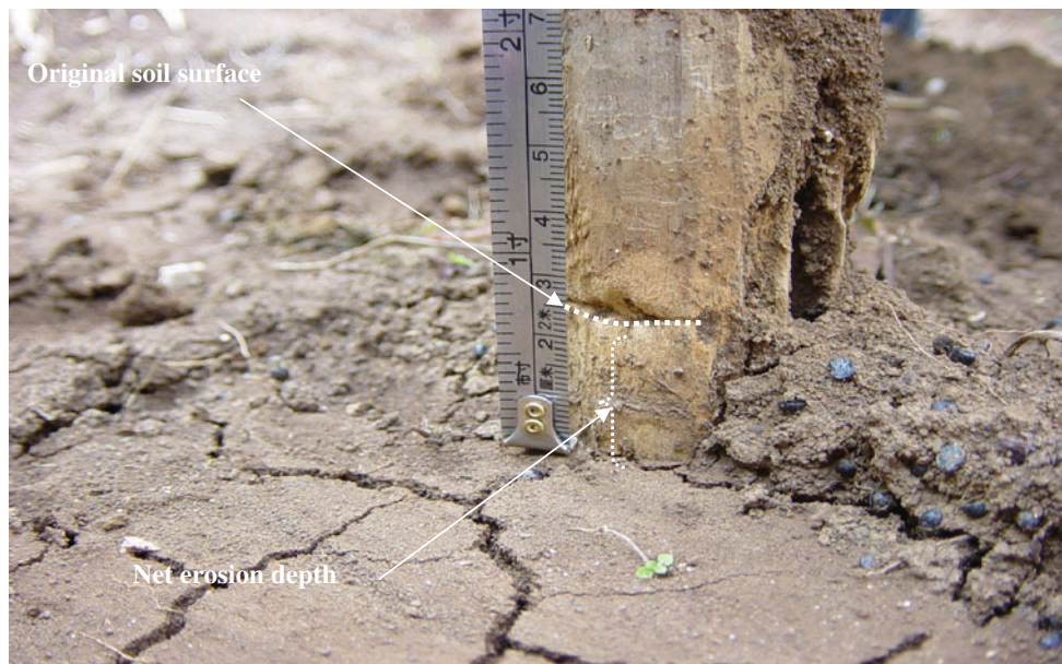
Fig. 4 Soil erosion recorded by stake-driven method
