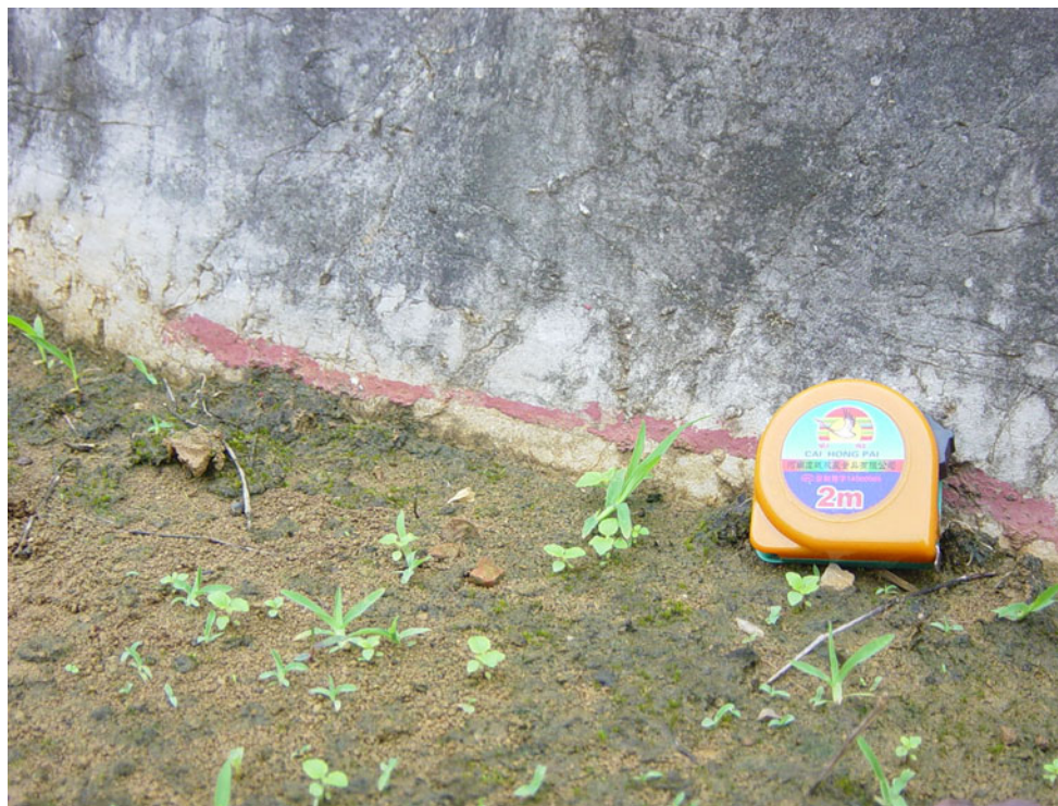
Fig. 5 The soil loss measured by line-drawing method
