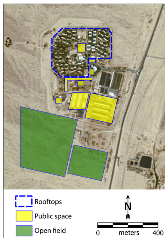
Fig. 9. Available areas for PV deployment in Kibbutz Ketura.
