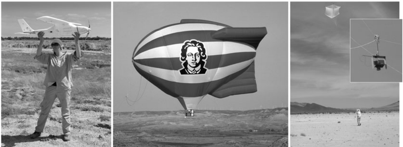
Figure 2. Platforms used for gully monitoring with small-format aerial photography. (left) Auto-piloted model airplane (wingspan is 1.6 m; kindly provided by MAVinci); (centre) hot-air blimp (length is 11 m) with double camera system; (right) large rokkaku-type kite (height is 2.5 m) with camera sledge.
