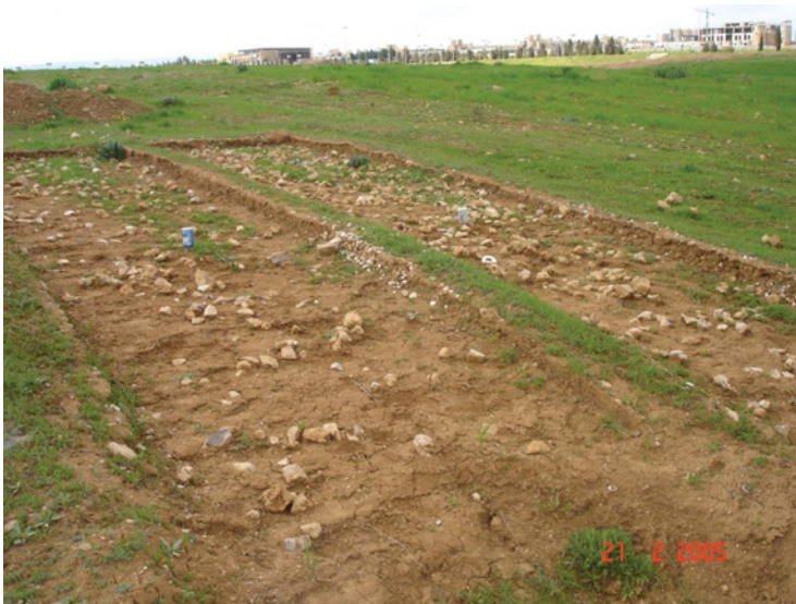
Figure 1. General view for the experimental plots; the 15% stone cover plot is shown in the right and the 5% stone cover plot is on the left.
